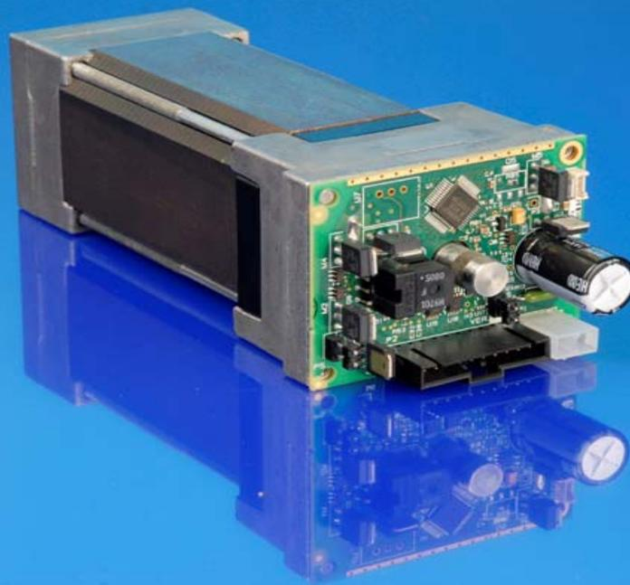
This manual was developed as a guide for use by FIRST Robotics Teams using Controller Part Number 840205-000 in conjunction with the Nidec Dynamo BLDC Motor.
