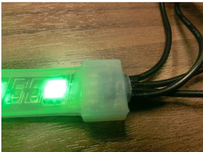
4. When the furthest wire over from the 12V wire is attached to a power source, you should see GREEN lights.
