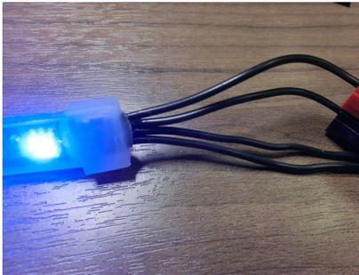
2. When the cable adjacent to 12V wire is attached to a power source, you should see BLUE lights
