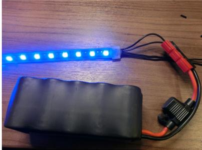
1. Using a 12V battery, you can check your setup by plugging the 12V line into positive 12V power and another cable to ground.
