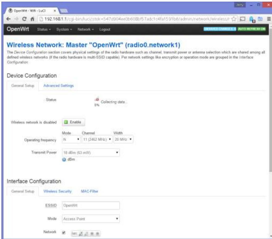
3. Under 'Interface Configuration' you can change your SSID to your team number (in this example we are using team 9999), if you wish to make this a secure connection, you can click on the 'Wireless Security' tab and use your desired encryption. Click on 'Save & Apply' at the bottom of the page.
