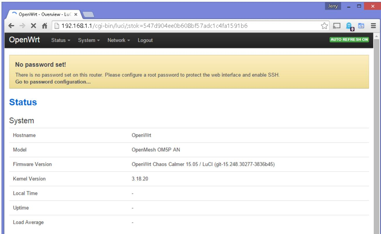
3. Click on the "Go to password configuration" at the top in the yellow box to set a password and remove the warning.
