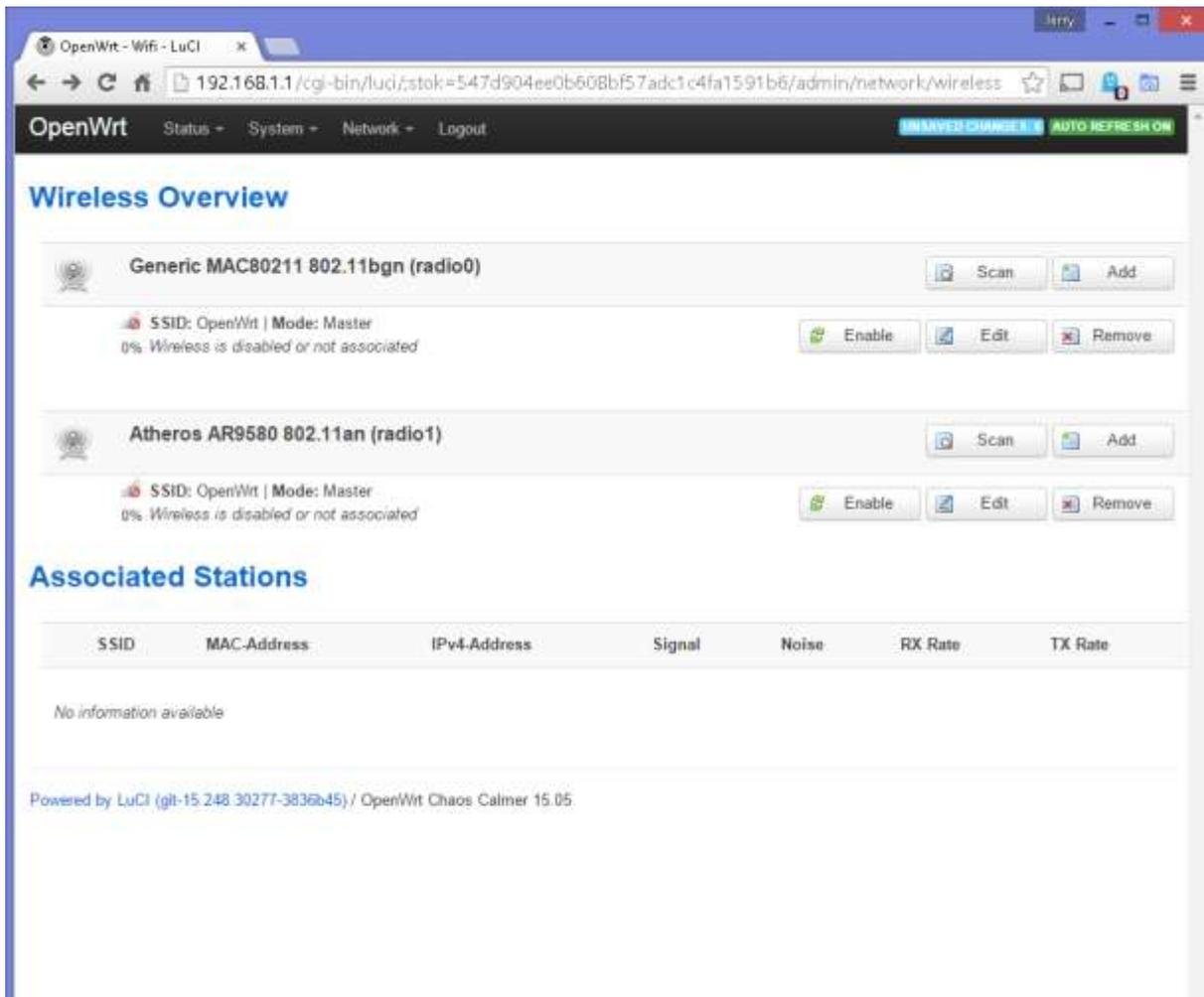
2. The 802.11bgn (radio0) is the 2.4GHz WiFi, 802.11an (radio1) is the 5GHz WiFi. Click on Edit next to the (radio0)
